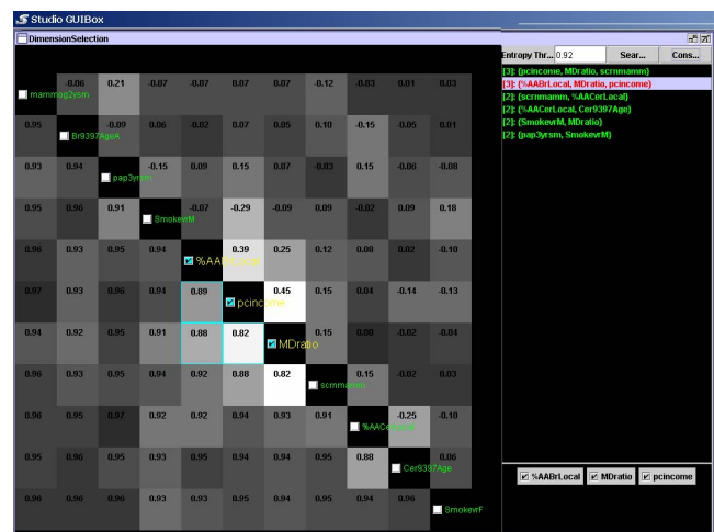
Figure 5. Dimension selection tool. Conditional entropy values (below diagonal) and correlation values (above diagonal).
